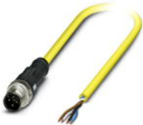
Sensor/Actuator cable, 4-position, TPE, yellow RAL 1021, Plug straight M12 SPEEDCON, A-coded, on free cable end, Cable length: 2 m
